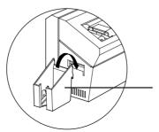
Install Card Output Hopper onto printer by hooking over bottom edge of card exit aperture.
